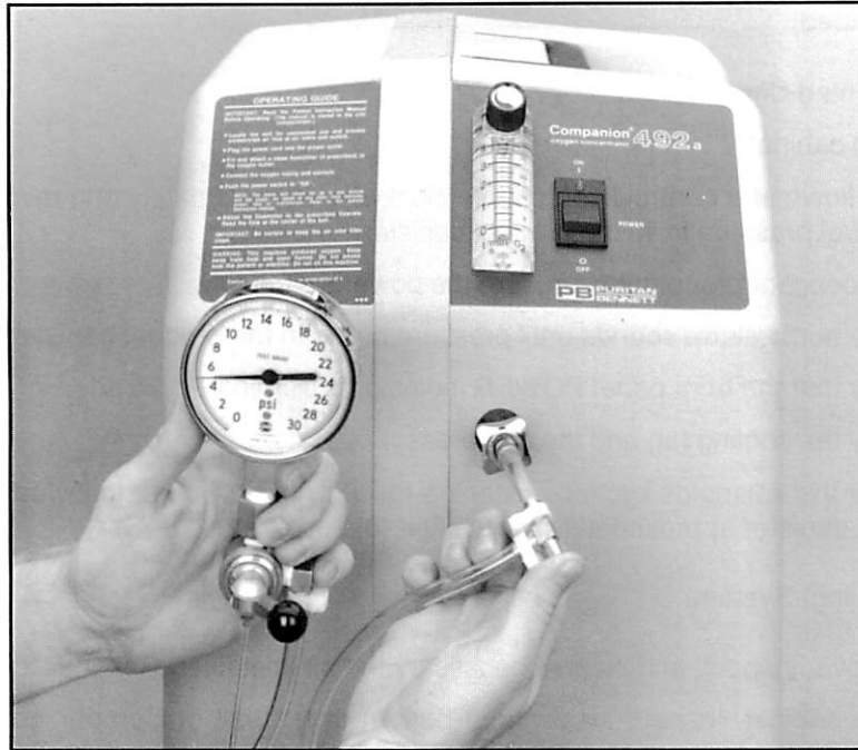
Figure 3-5: Outlet Pressure Testing
